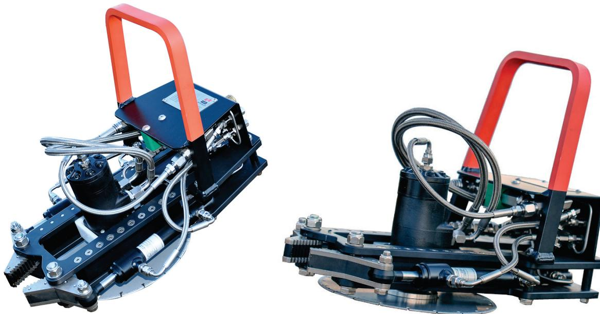
The IKM Technology manipulator held **Subsea Saw** has a long track record. It is designed to cut steel pipes, steel profiles, wires and chains up to 90mm.
