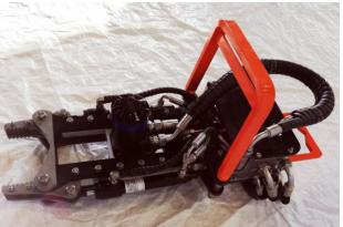
The IKM Technology manipulator held **Subsea Saw** has a long track record. It is designed to cut steel pipes, steel profiles, flexirisers and chains from 30mm up to 120mm.
