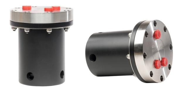
The IKM Subsea **Subsea Compensator 0,3 Liter** is a general-purpose compensator for underwater hydraulic systems. It provides a given volume and pressure for oil-filled subsea equipment. A mechanical oil level indicator pin comes out when it is filled with oil. It can be installed both vertically and horizontally.
