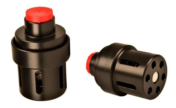
The IKM Subsea **Subsea Compensator 30 Milliliter** is a general-purpose compensator for underwater hydraulic systems. It provides a given volume and pressure for oil-filled subsea equipment. A mechanical oil level indicator pin comes out when it is filled with oil. It can be installed both vertically and horizontally.
