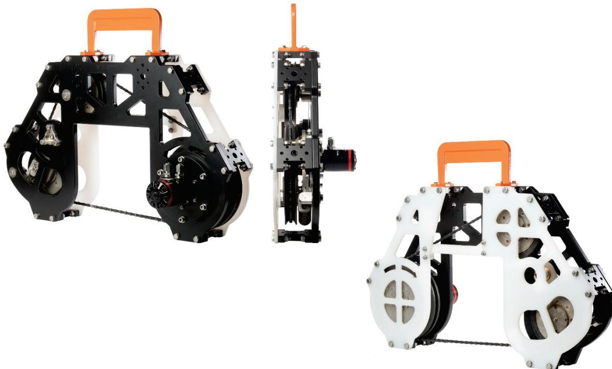
The IKM Technology manipulator held **Subsea Saw** has a long track record. It is designed to cut steel pipes, steel profiles, wires and chains up to 320mm. The diamond wire saw is used for various cutting operations where conventional rotating blades are insufficient. The saw has exceptional performance and a long service life.
