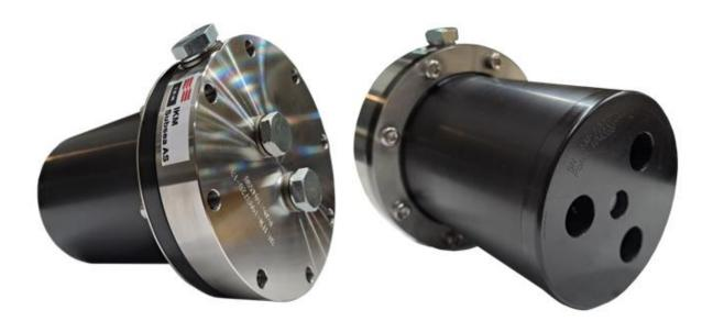
The IKM Subsea **Subsea Compensator 0,25 Liter** is a general-purpose compensator for underwater hydraulic systems. It provides a given volume and pressure for oil-filled subsea equipment. A mechanical oil level indicator pin comes out when it is filled with oil. It can be installed both vertically and horizontally.
