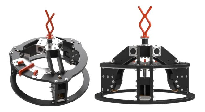
The IKM Subsea **Subsea AV/AX Mechanical Ring Tool** for removal/installation of AX/VX gaskets is a mechanical tool with no requirement for hydraulic or electric supply from an ROV. This gives the operator the option to transport the tool to/from the worksite without recovery of the ROV. Suitable for use with or without tubing hanger installed in the wellhead.
