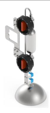
The IKM Subsea **Mini Gas Sampling Unit** is designed with ROV friendly grabbing bars and valve handles. The top valve opens for gas into the sample tank and the bottom valve vents out to sea so that operators can see when the gas sample bottle is full. The sample can be transferred from this unit to smaller 500 cc sample bottles (IKM-1048787) when the unit is on deck. Available for rent.
