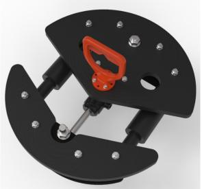
The IKM Subsea AX-VX Gasket Tool Hydraulic is designed to give the operator an effective and simple method of removing/installing an AX- or VX-Gasket by use of an ROV. A spring-loaded failsafe assembly, together with the lower locking plate in the sandwich assembly ensures that the AX- or VX-Gasket cannot be lost/dropped out of the tool by accident. The tool must be hydraulically operated to unlock and release the gasket.
