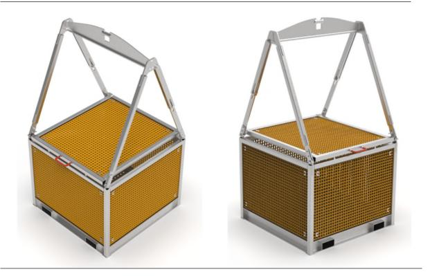
The IKM Subsea **Subsea Basket** is designed for subsea lifting of tools and equipment. It is a lightweight structure made out of stainless steel and grating. Foldable lifting yoke for easy access during loading and unloading. The lid is locked when the yoke is in a lifting position, and can also be removed if required.
