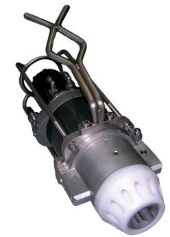
Thus in the case of a loss of hydraulic power the wings will release. The tool uses a high specification drive motor for consistent torque output characteristics, even if used with direct hydraulic pressure control without the feedback sensor. The motor shares casing oil with the gearbox therefore avoiding the need for a separate compensator.
