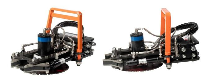
The IKM Subsea manipulator held **Subsea Saw** has a long track record. It is designed to cut steel pipes, steel profiles, flexible risers/cables and chains up to 115 mm.
