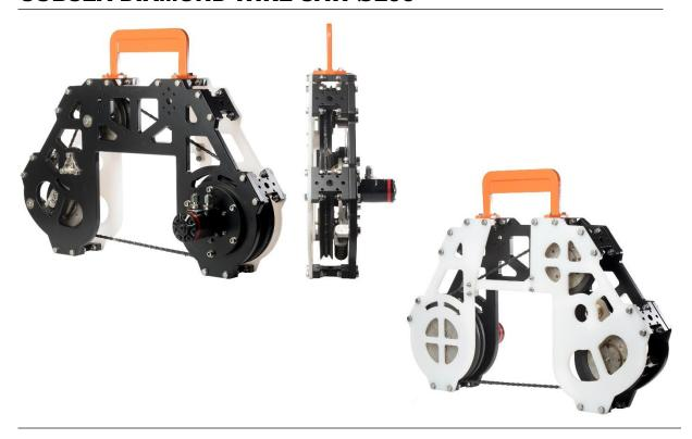
The IKM Subsea manipulator held **Subsea Diamond Wire Saw** has a long track record. It is designed to cut steel pipes, profiles, wires and chains up to 290 mm. The diamond wire saw is used for various cutting operations where conventional rotating blades are insufficient. The saw has exceptional performance and a long service life.
