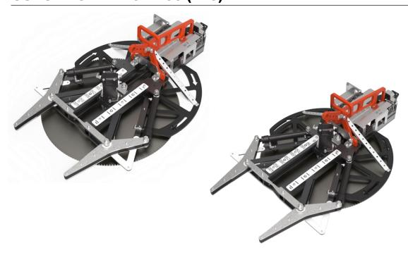
The IKM Subsea manipulator held **Subsea Saw** has a long track record. It is designed to cut steel pipes, profiles, chains, armored cables and flexible risers up to 425 mm. The saw has a clamp and an automatic feed function on the sawblade.
